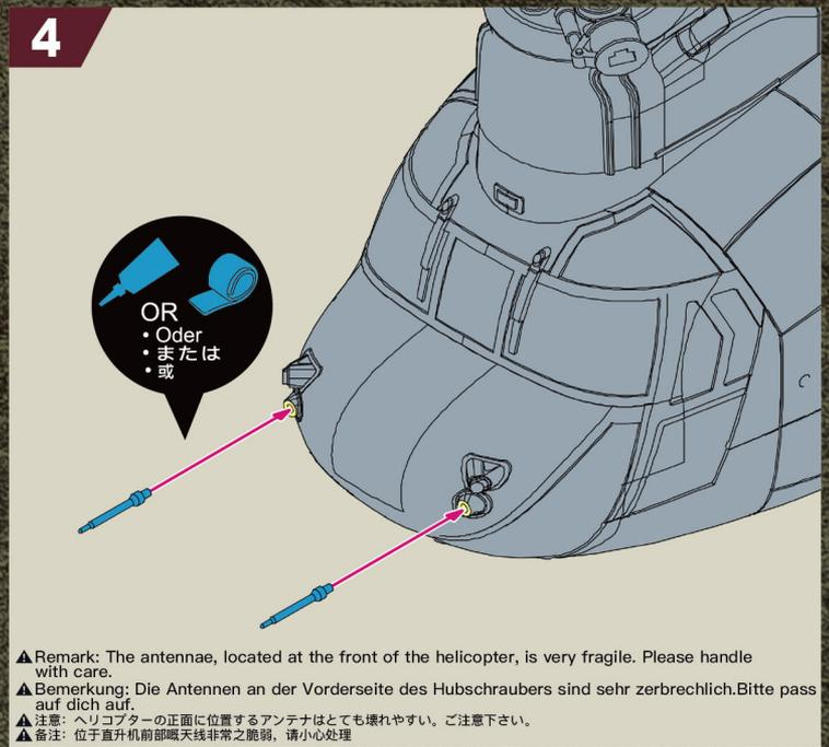
▲ Remark: Please use a tiny amount of glue or adhesive to attach the two parts.
